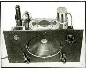
Fig. A. The front-panel appearance of the interphone.
